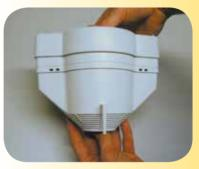
Choose the height of the box according to the depth of the spotlight to be installed, the box and the average dimensions (the most common). It is however possible to obtain a 3cm higher box by simply moving the cover higher. This will allow installation of spotlights up to 120mm in depth.
