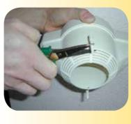
Choose the diameter of the next spotlight to be installed. If you do not know the diameter, do as follows: find out, according to the dimensions of the area or to the tastes of the client if the spotlight will need to be small, medium or
